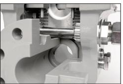
With orifice plate out of flow line
