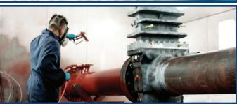
Canalta applies a standard coating to all Dual Chamber Orifice Fittings that includes a non-lift oxide primer and fast-drying enamel finish in Canalta Grey and burgundy top. Custom coatings for special environments - including maritime, humid, high temperature and others - custom colours and primer only applications are also available.
