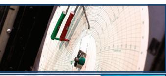
Our comprehensive **Quality Management System** includes full function, hydrostatic and pneumatic pressure testing to prevent imperfect fittings from reaching service. Standard testing comes at no extra charge and includes verifiable pressurization to 150% of working pressure. Additional inspections - such as radiography, ultra sonic and liquid dye penetration - are also available.
