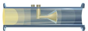
The centrally-located cone directs flow to the outside wall, effectively conditioning disrupted flows.
