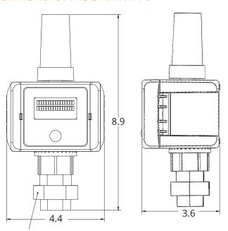
1" NPT Female Thread Union Coupling STD 2-PIN Pickup Connector Included
