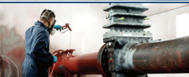
Canalta applies a standard coating to all Dual Chamber Orifice Fittings that includes a non-lift oxide primer and fast-drying enamel finish in Canalta Grey and burgundy top. Custom coatings for special environments - including maritime, humid, high temperature and others - custom colours and primer only applications are also available.
